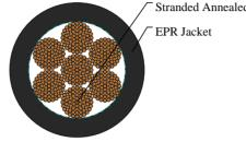
Stranded Annealed Copper Conductor
